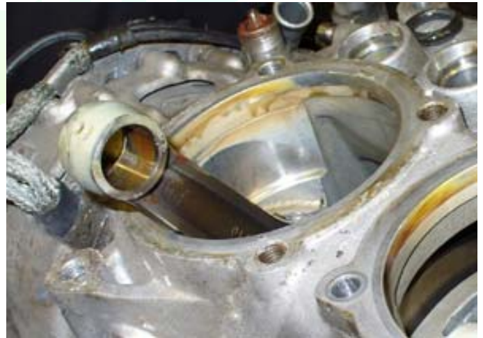
Figure 9: White lead deposits from Avgas on top of conrod
