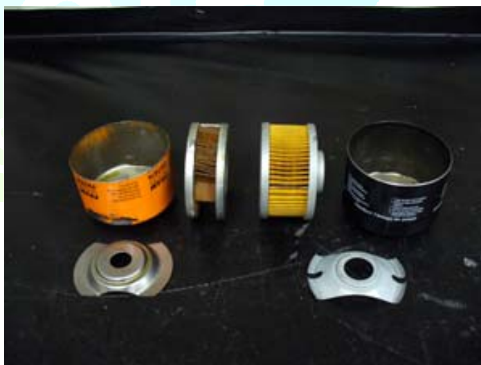
Figure 26: Genuine filter and pattern one. Pattern filter is on left with much smaller filter area.
