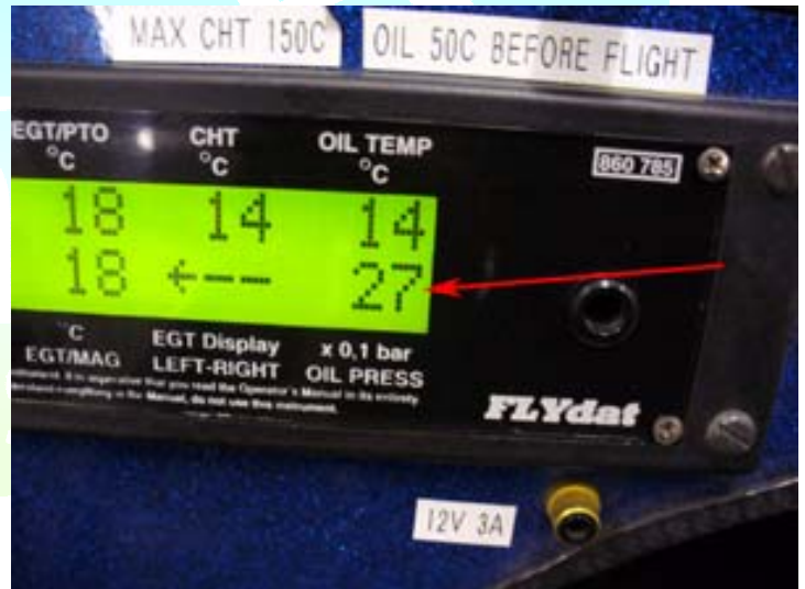
Figure 21: Flydat showing 2.7 bar oil pressure
