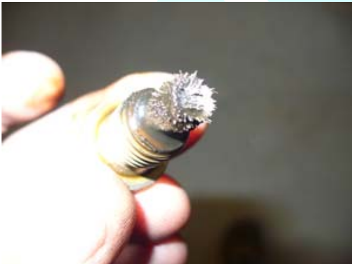
Figure 29: furred magnetic plug before cleaning
