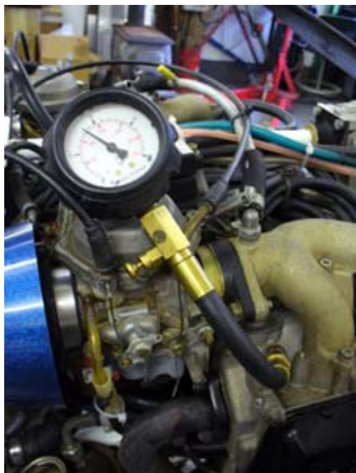
Figure 50: Conventional automotive style compression tester for fault finding
