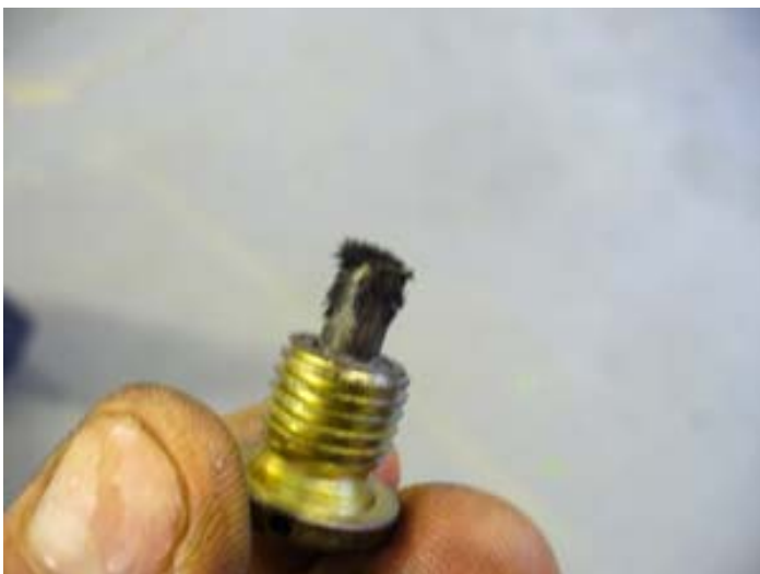
Figure 31: Plug after cleaning in carb cleaner
