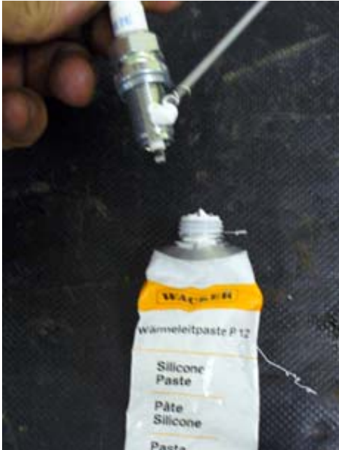
Figure 32: Applying heat sink paste
