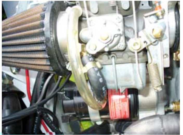
Figure 35: Typically modified vent tube that could affect mixture, (sprung closed throttle system)
