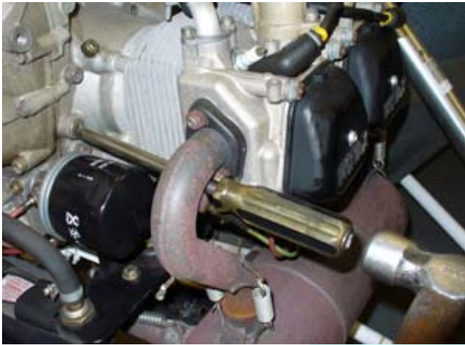
Figure 27: Clouting the magnetic plug to free it off
