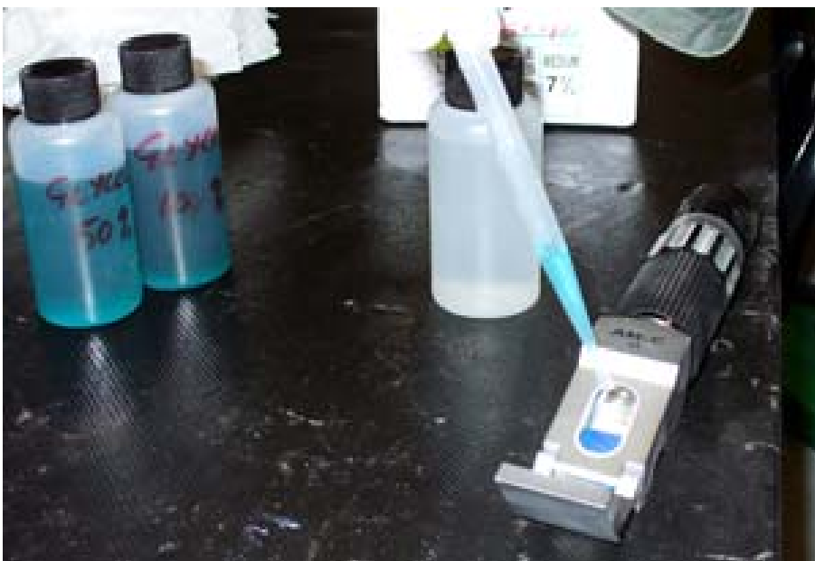
Figure 14: Using refractometer to check glycol ratio
