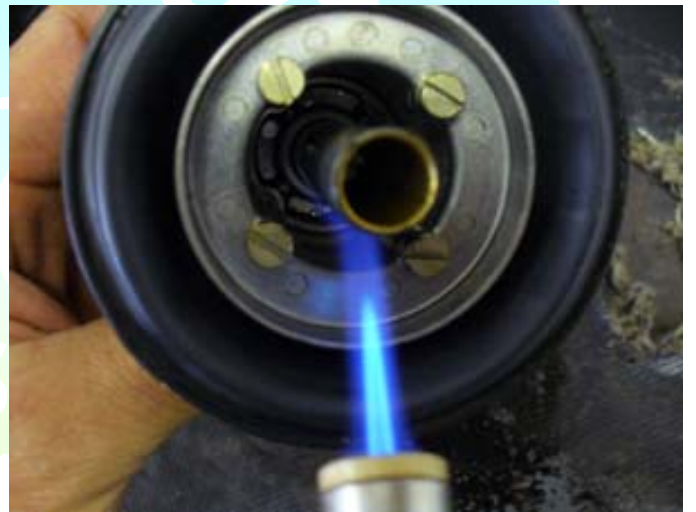
Figure 37: softening Loctite by applying heat to remove carb needle
