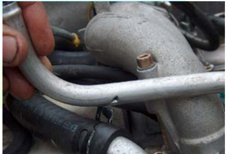
Figure 13: Oil tube worn through on hose clamp
