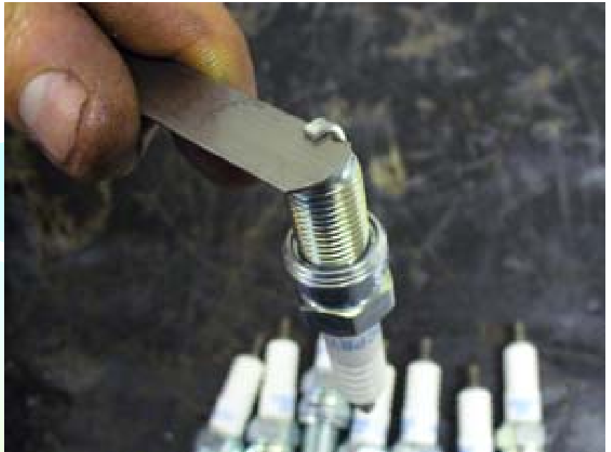
Figure 33: Checking plug gaps before installation
