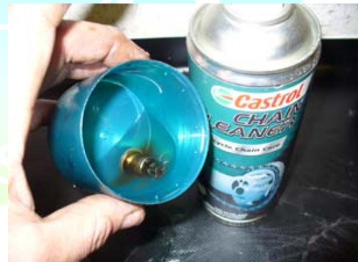
Figure 30: Cleaning magnetic plug
