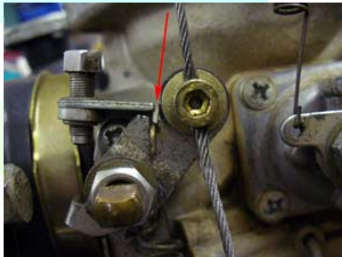
Figure 42b: Throttle lever with clearance at full throttle
