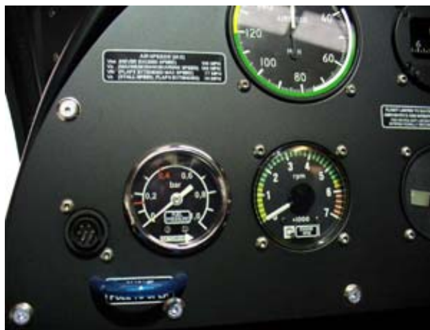
Figure 11: Fuel pressure gauge fitted
