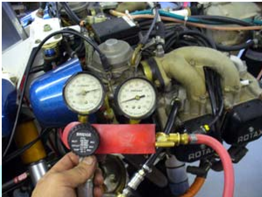
Figure 51: Leak down (differential) compression tester to be used during Maintenance
