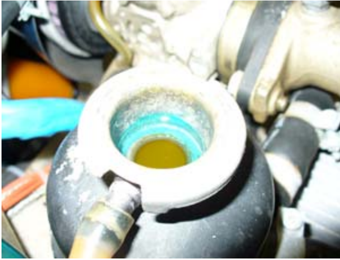
Figure 16: Corroded expansion tank
