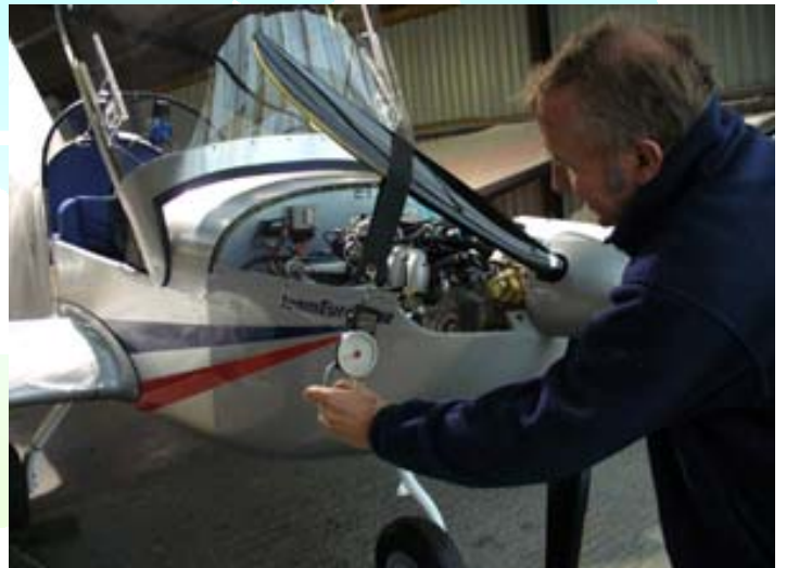
Figure 49: measuring friction torque at ½ m on the prop
