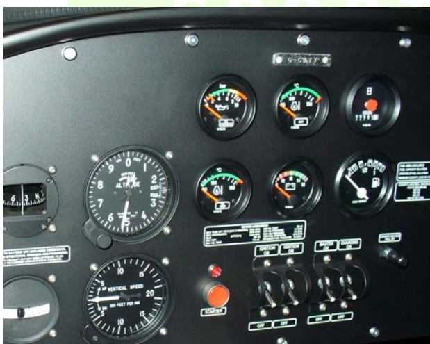
Figure 3: Instrument marking kit fitted to a Eurostar
