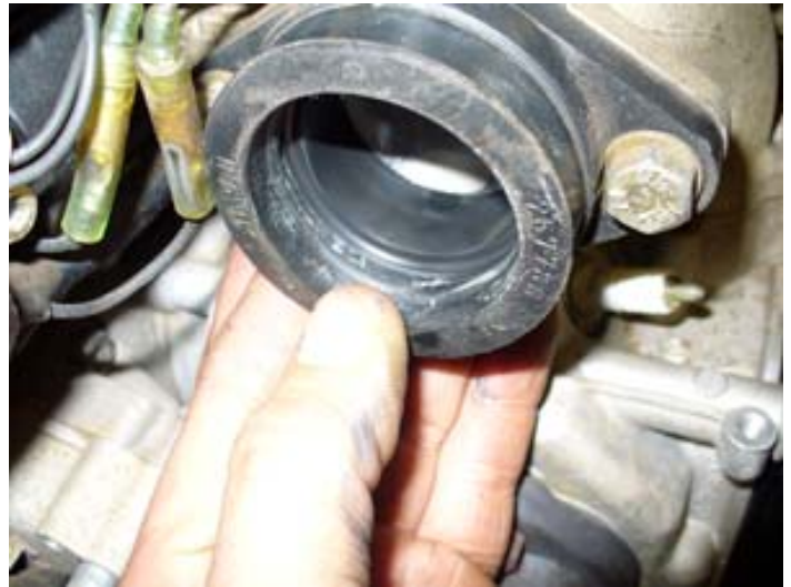
Figure 39: Checking carb rubber flange for cracks
