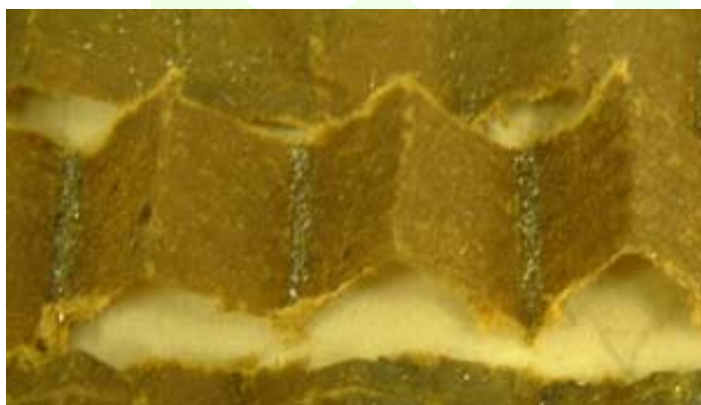
Figure 25: Contaminated filter papers (This engine needed further investigation)
