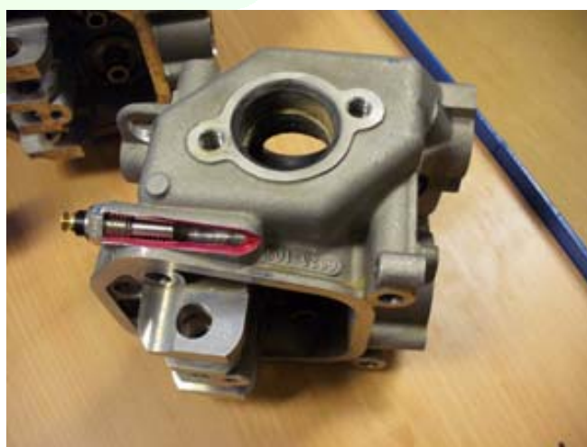
Figure 4: Cylinder head temp probe on cylinders 2/4 (not water temp)
