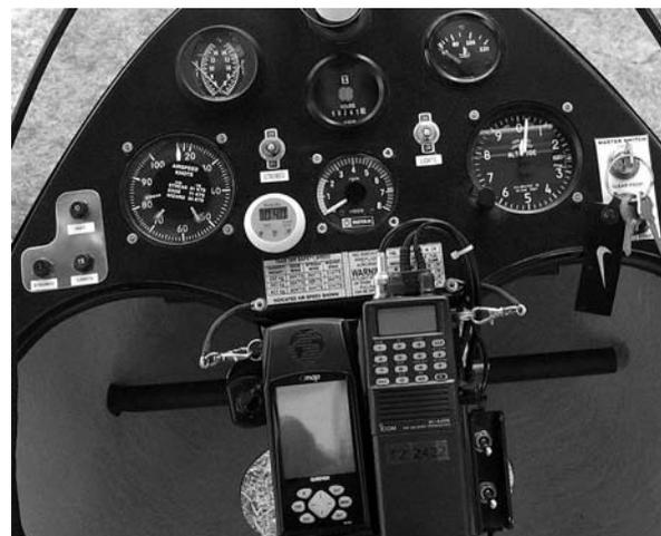
Note: Lanyards on radio and GPS and correct labelling and orientation of switches
